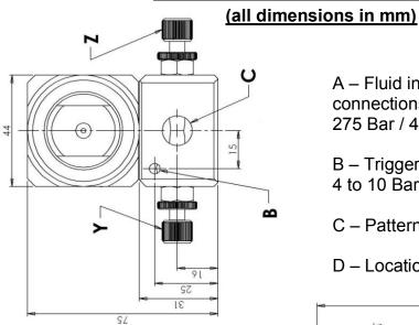
A – Fluid inlet 1/4" NPS (x2) (see fluid connections & options 275 Bar / 4000 psi Maximum
